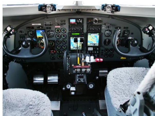
The BT-67 has a new digital "glass cockpit" in place of the old C-47 panel.
