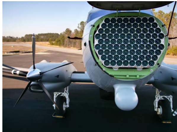
The RAPTR telemetry antenna fills the aircraft nose. The weather radar formerly located here has been moved to the bulbous chin housing below.
