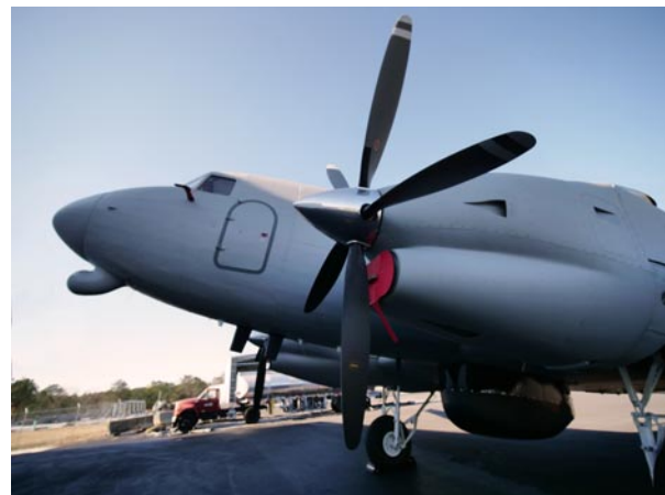
Modern turboprop engines take the place of the radial piston engines that powered the C-47 and DC-3. The fuselage was lengthened 42 inches directly behind the cockpit for more interior space and to keep the crew compartment ahead of the new propellers on the turboprop engines, which extend farther forward than the old piston engines.
